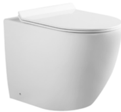
TCT 02E FLOOR STANDING TOILET Size: 540x365x400mm Washdown / P-trap, 180mm roughing-in
