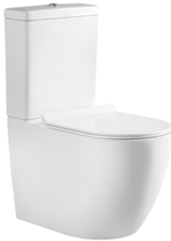
TCT 02B TWO-PIECE TOILET Size: 680x370x830mm Washdown / P-trap, 180mm roughing-in
