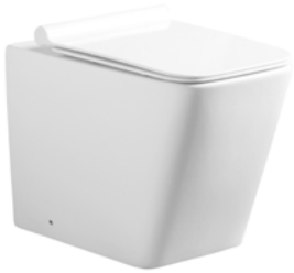
TCT 03E FLOOR STANDING TOILET Size: 555x355x410mm Washdown / P-trap, 180mm roughing-in
