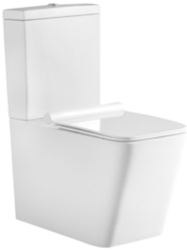
TCT 03B TWO-PIECE TOILET Size: 665x385x835mm Washdown / P-trap, 180mm roughing-in
