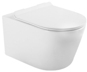
TCT 01F WALL HUNG TOILET Size: 535x365x310mm Washdown / P-trap, 180mm roughing-in
